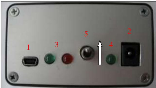
*Controller front; switch in NORMAL position*
