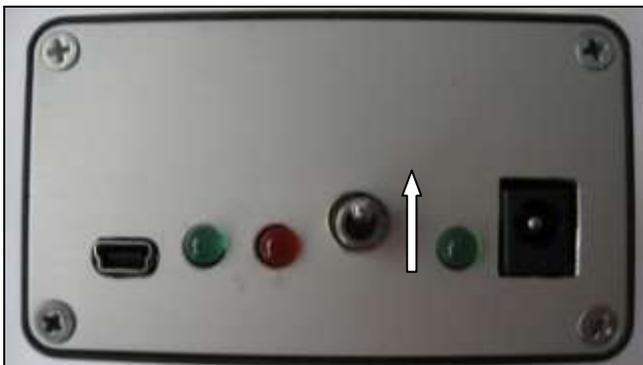
Controller front; switch in NORMAL position
